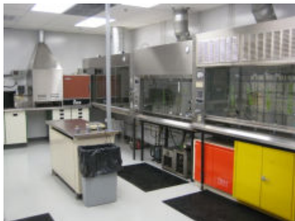
Fume Hoods, Fischer Assay and Distillation Apparatus, and Drying & Muffle Furnaces
