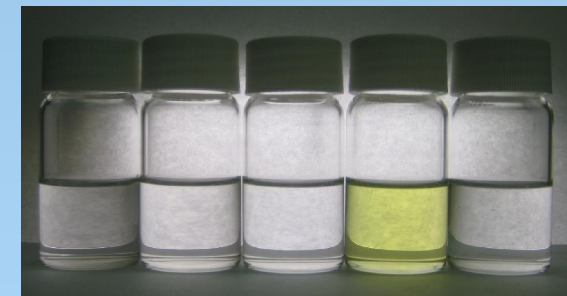
Boiling Point Fractions After Pilot Hydrotreating - Naphtha, Jet/Kero, Diesel, Gas Oil, Light Oil -
